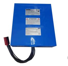
Lithium-Battery Pack with protection electronics (BMS single cells monitoring), protects the battery against overcharge, deep discharge and short circuit, Implemented cell balancing, with BMS-interface for service purposes (number of cycles, capacity, temperature, etc.)
